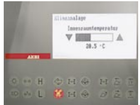
On the keyboard to the right next to the lever, the driver can operate the electronics menu, which is displayed on the screen (in one of four possible languages). Values critical to the operating state are immediately and clearly displayed on the screen.
