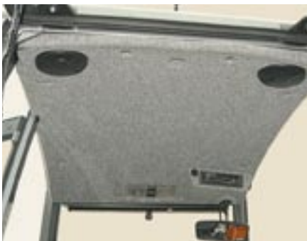
Cab roof with built-in radio and loudspeakers.
