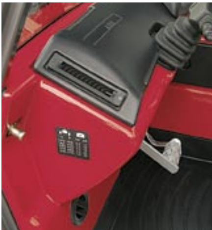
Blower aperture of the air-conditioning system fitted as standard.
