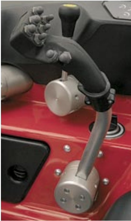
Using the multifunction control lever, the driver can operate a total of 20 functions with the same hand.
