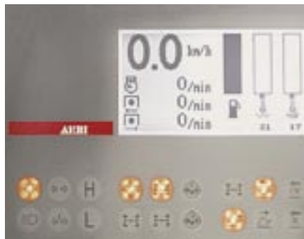
On the keyboard to the right next to the control lever, the driver can operate the electronics menu, which is displayed on the screen (in one of four possible languages). Values critical to the operating state are immediately and clearly displayed on the screen.
