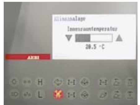
On the keyboard to the right next to the control lever, the driver can operate the electronics menu, which is displayed on the screen (in one of four possible languages). Values critical to the operating state are immediately and clearly displayed on the screen.
