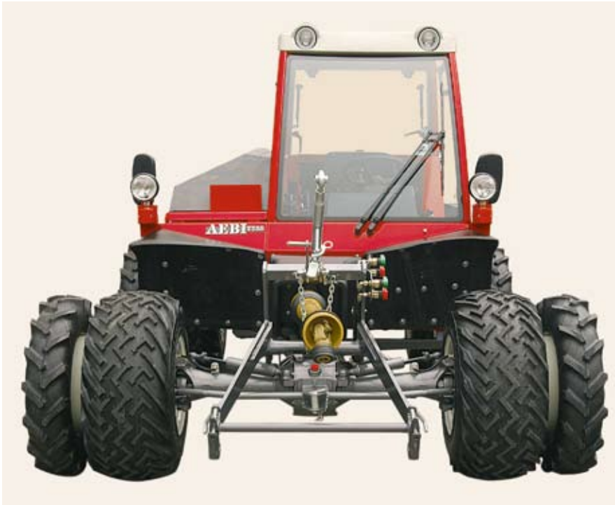
On the TT55, dual wheels can be fitted on the front axle as well as on the rear axle, without restricting the steering lock...
