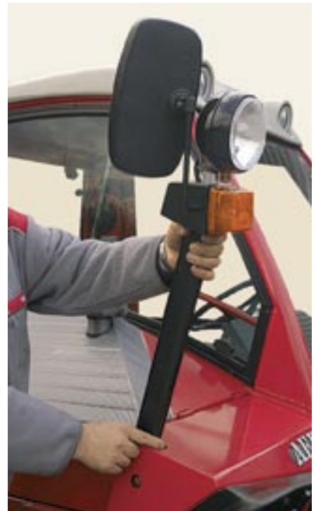
The height of the headlights can be adjusted, or if necessary they can be removed.
