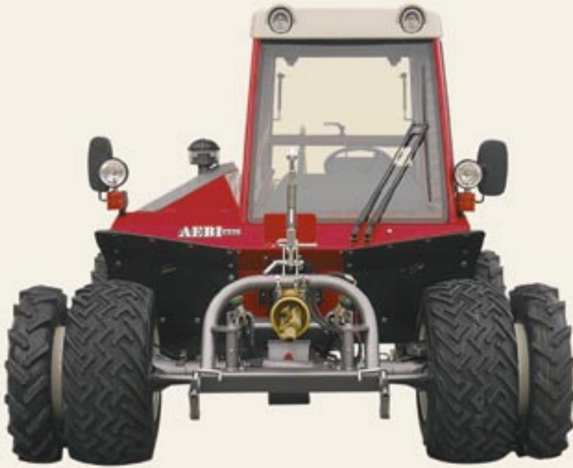
The highly manoeuvrable TT75 causes minimum damage to the ground. Large-size low-pressure tyres with a large footprint mean extremely low ground pressure.
