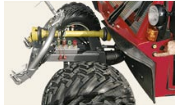
The three-point front lifting mechanism for universal implement attachment, with practical and time-saving external operation.
