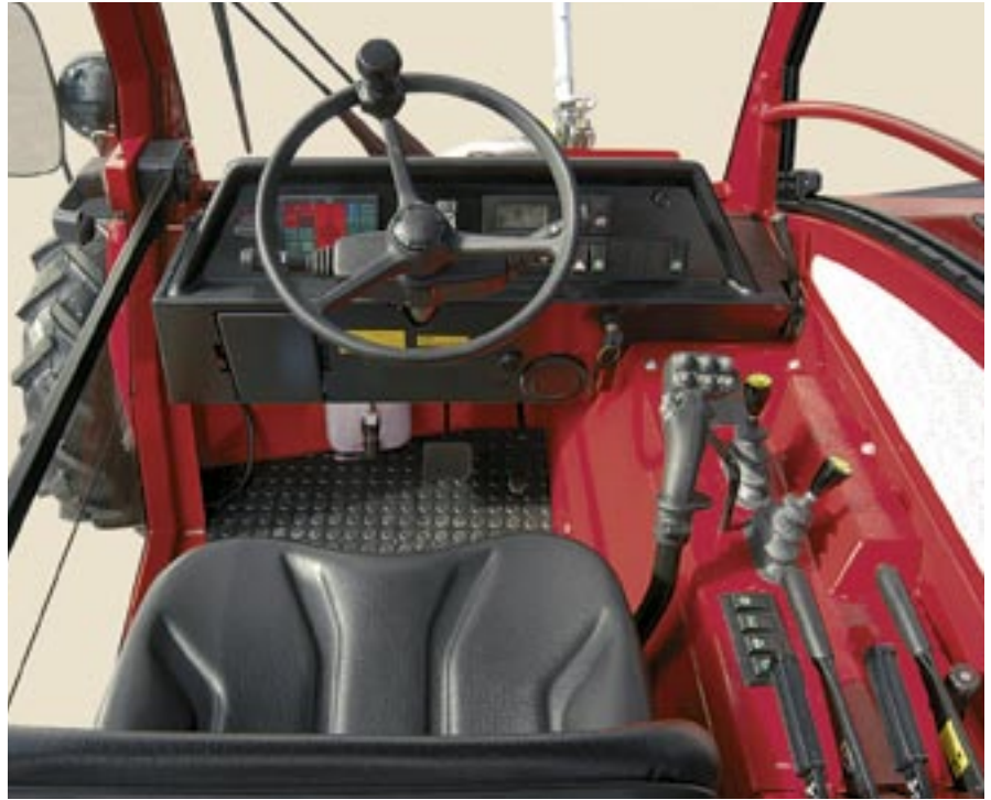
The very roomy cockpit, insulated against vibration and noise, with a curved front screen and clearly laid out indicator instruments, also provides excellent all-round visibility.
