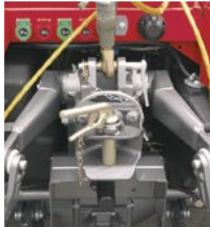
Many additional hydraulic connections and a trailer-hitch with rapid adjustment.
