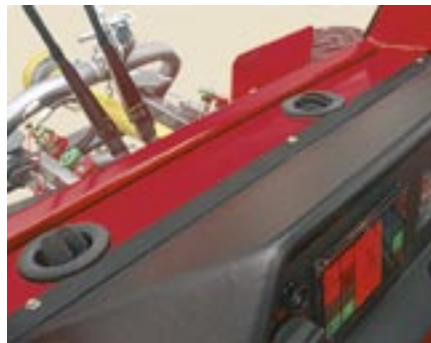
Output openings of the front-screen defrosting system.
