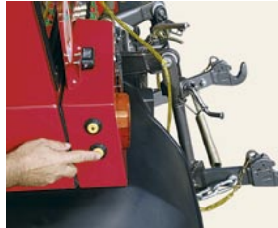
Convenient external operation of the rear lifting mechanism makes it easier to raise and lower the implements carefully.
