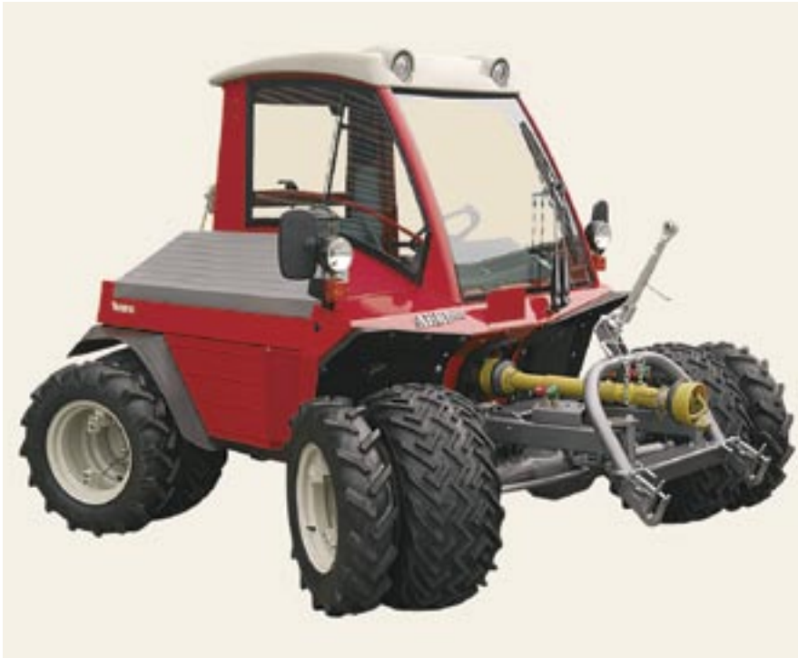
Modern and elegant: the Terratrac Aebi TT75 implement carrier, with hydrostatic operation and four-wheel steering.
