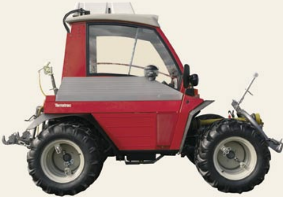
Thanks to its light weight, low centre of gravity and almost square wheel base, this Terratrac is particularly suitable for use on steeply sloping ground.
