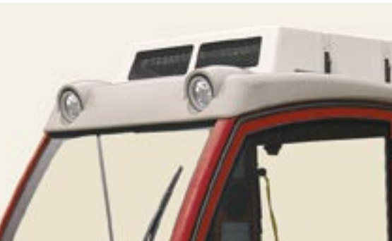
Working headlights built into the reinforced plastic roof.
