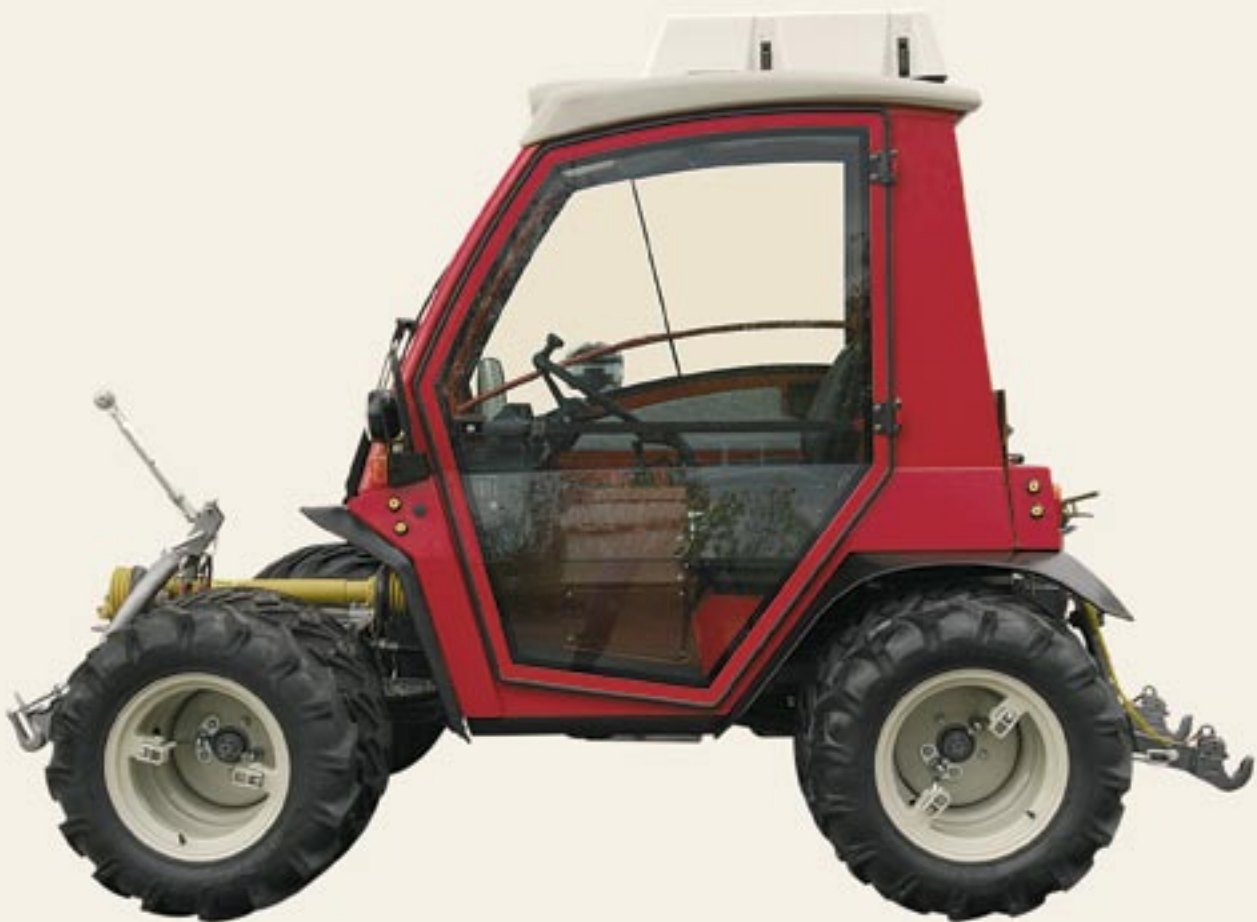
Not a luxury for a professional work-station. As an option: all-round-view cab with heater/defrosting system or air-conditioning with dust/pollutant filter.
