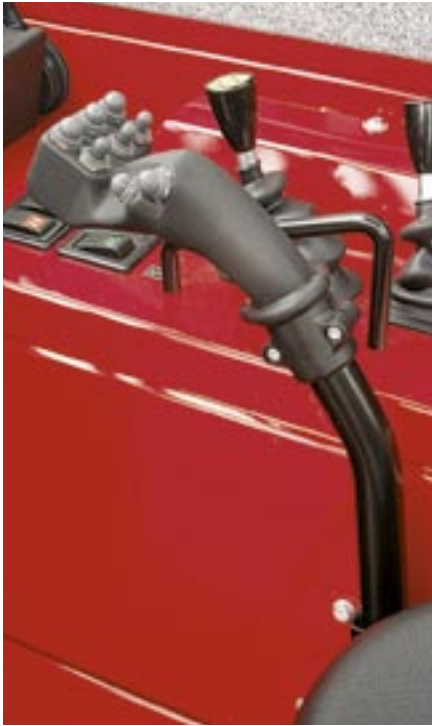
All important functions under control: using the multi-function control lever, adjust the continuously-variable speed precisely, pre-select the drive mode and engage the differential locks.
