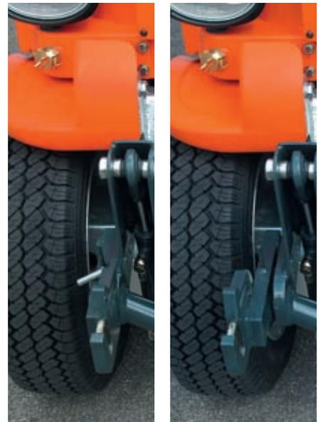
**Flexible implement connection:** The 3-point front hydraulic lift (Cat. I) can be adjusted rapidly to suit the available Rasant implements.
