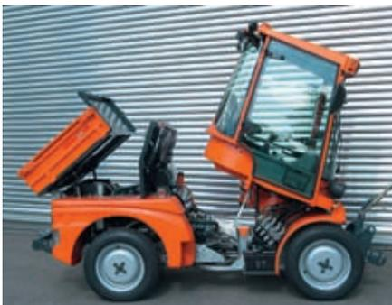
**The driver's cab, which offers the best possible visibility, is not only air-conditioned but is also soundproofed. In addition, like the loading platform it can also be tilted in order to give free access to the various points for servicing work.**
