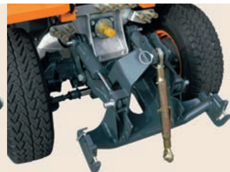
Front and rear three-point, Cat. I hydraulic linkage with implement weight transfer and the Aebi quick-fit implement connecting system. The power take-off drive (PTO), which can be engaged under load, can function at various speeds on both sides.
