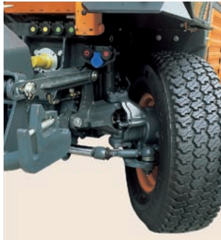
Dual-level, jib-axle gearbox at front and rear. Hence the large ground clearance of 28 cm.
