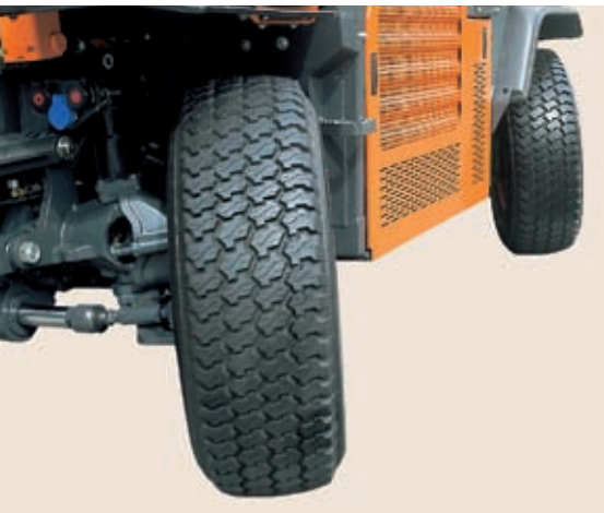
Dual-level, jib-axle gearbox at front and rear. Hence the large ground clearance of 28 cm.
