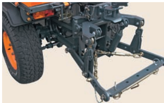
Front and rear three-point, Cat. I hydraulic linkage with implement weight transfer and the Aebi quick-fit implement connecting system. The power take-off drive (PTO), which can be engaged under load, can function at various speeds on both sides.
