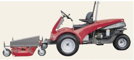
Functionality with system. Implement carrier and implement form a single unit and are ideally matched. Rotary deck mower, flail mower, cutter bar, sweeping brush, snow clearing devices and other implements are connected in no time at all thanks to the Aebi quick-fit connector system (also existing Aebi single-axle machine implements).
