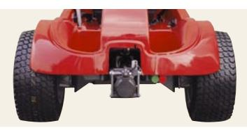
Depending on the actual application, Terra tyres or turf tyres can be used, and at the front double wheels. By reversing the front wheels, the vehicle width can be reduced from 130 to 110 cm, with double tyres the width can be increased to 160 cm.
