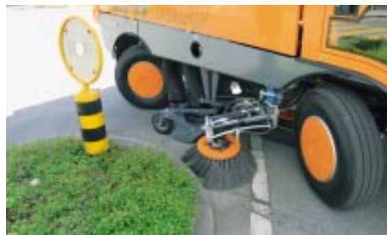
Hugs corners: Thanks to its four-wheel steering, it has a minimum sweeping radius of 67 cm.
