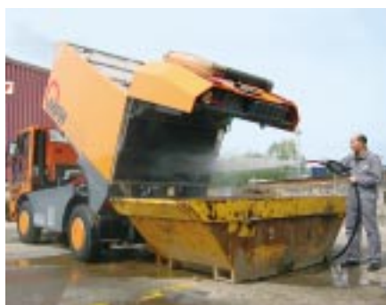
The Aebi MFH 5000 cleans containers, façades, signs, etc. at high pressure.
