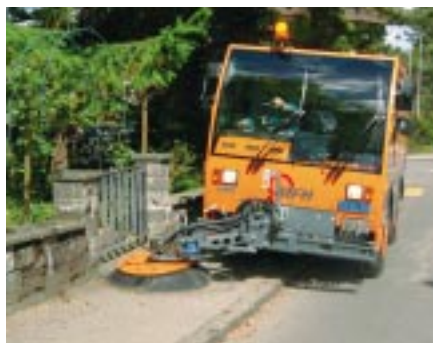
The sweeper can drive and work on staggered levels along narrow pavements.
