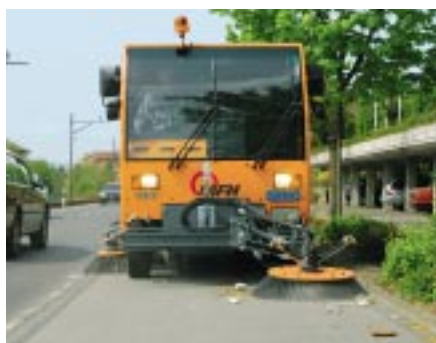
Wide working range: The front brush can be extended on either side and has a cleaning swathe ranging from just 90 cm to as much as 290 cm.
