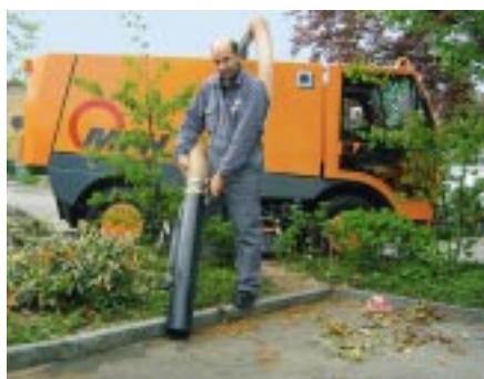
Highly effective (suction): Handheld suction hose for thick foliage and for gullies.
