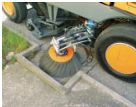
Optimum recess cleaning: The side brush can be extended and is hydraulically adjustable.
