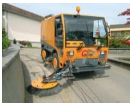
The front brush can be mounted on the shoulder and sweep the road at the same time. Not every sweeper can do that...
