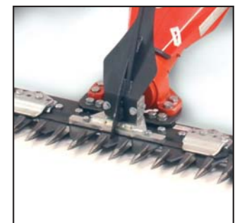
Disengageable, silent running planetary mower drive with overload protection
