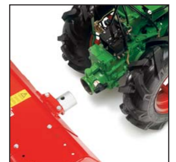
Quick-fit connection system for tool-less implement change
