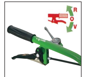
Safe reversing, both hands stay on the handlebar
