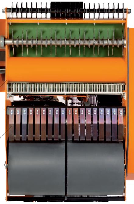
The rollers the Overseeder travels on then very gently close the top of the groove without compacting the subsoil that has just been cut open. This places the grass seed in a cocoon, so that is protected and allowed to germinate.
