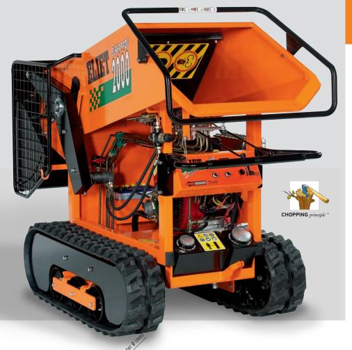
Resist ™ knives V-belt Multi-purpose grating SUPER prof 2000 18/13.2 Option ABM \*\* 24 HS Steel\* XPB 2360 Wheel drive | 1.830 x 835 x 1.380 | 355 Grating with holes 30-35 mm toothed roller 23 "/min V-belt Speed controller for infeed roller CROSS COUNTRY 18 - 13,2 | 120 480 XPB 2360 toothed roller 23 m/min ABM-system Track drive | 1.830 x 900 x 1.330 | 420 24 HS Steel \* Conveyer (length 2/1,4 m) Trailer for quick transport \* reversable
