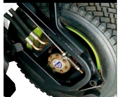
NO REAR AXLE, HYDRAULIC WHEEL MOTORS
