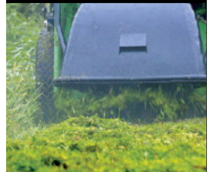
TALL GRASS CUTTING WITH HYDRAULICALLY CONTROLLED DEFLECTOR
