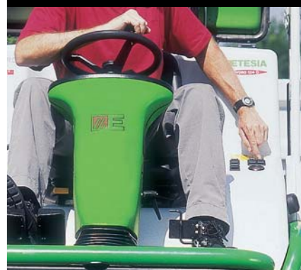
EMPTYING FROM THE OPERATOR'S SEAT
