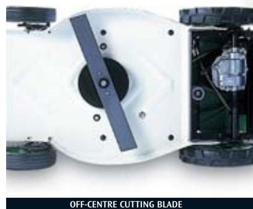
OFF-CENTRE CUTTING BLADE
