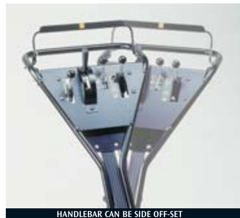
HANDLEBAR CAN BE SIDE OFF-SET
