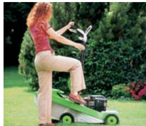
FOOT OPERATED RAISING OF THE HANDLEBARS
