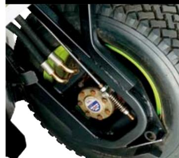
NESSUN ASSALE POSTERIORE, TRASMISSIONE MEDIANTE MOTORI SULLE RUOTE
