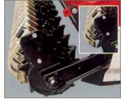
Rullo paker/ Raschiatore regolabile. Paker roller/ Adjustable scraper. Rouleau paker/ Racleur réglable. Paker-Walze/einstellbarer Schaber.
