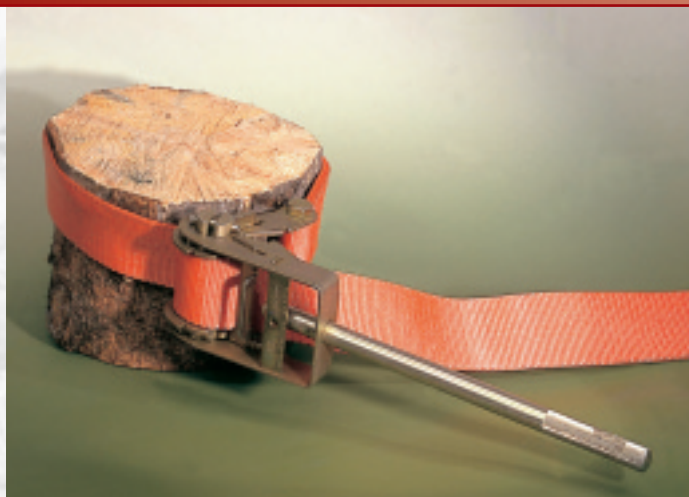
Trunk press. Prevents splitting of trunks under stress when felling or cutting them. Easy to use, with strong ratchet (breaking load 20 tons), length 4 m, belt width 75 mm, complete with tensioning lever ord.-no. 40200
