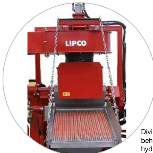
Dividing mesh 400 mm, stationary, electrical engine
