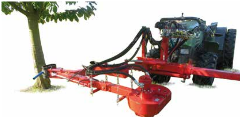
hydraulic and shaker unit for front attachment
