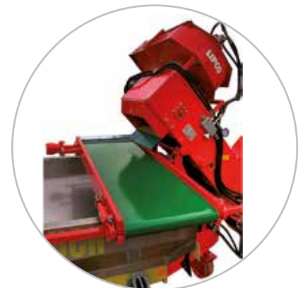
external filling of boxes (additional conveyor belt is mounted to 90°)
