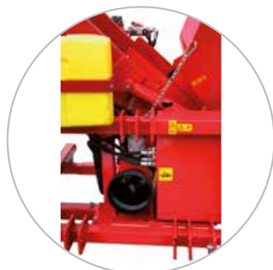
Photo shows proper hydraulic on FRD including oil cooler 12 V (optional, kit, for tractor that has an oil pump output of less than 40 l/min)
