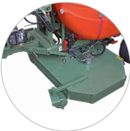
LIPCO under tree cultivator UBM 180/200/225 (hydraulic drive, 50-60 l/min oil quantity from tractor required)
