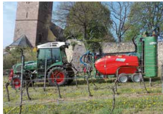
Photo: GSG-NV-VM2 with 1,500 l tank and tires 225/55-R12
