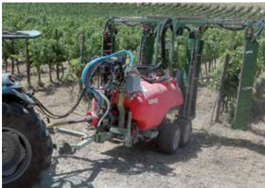
Photo: GSG-NV-VM2 with 2,000 l tank, with tires 23/10.50-12 8PR
