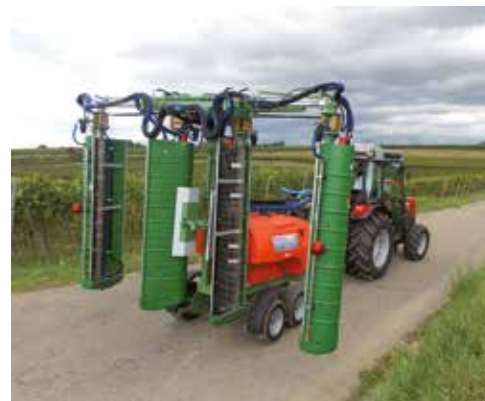
Photo: GSG-NV-VM2 with 600 l tank, with tires 195/55-R10C
