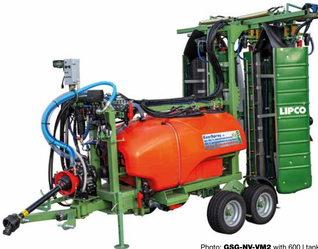
Photo: GSG-NV-VM2 with 600 l tank, with tires 195 R14C 8PR
