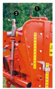
Achieve different spiking intensities by adjusting the entry angle of the tines.
